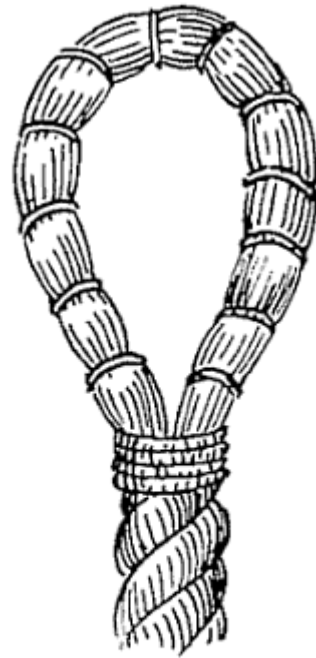
FIG. 90 B.—Flemish eye (complete).
