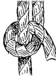
FIG. 30.—Lark's head with toggle (A).
