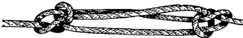
FIG. 82.—Sheepshank for free-ended rope.
