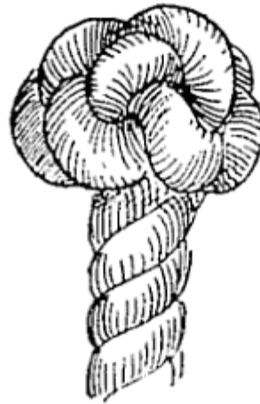
FIG. 125.—Wall crowned (complete).
