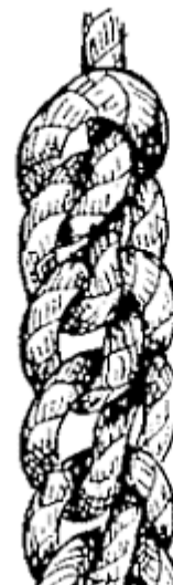
FIG. 70.—Single plait or monkey chain (making).
