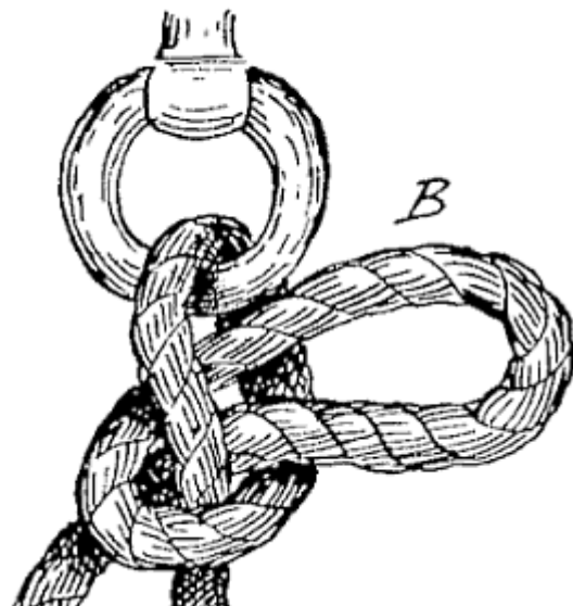
FIG. 31.—Lark's head with toggle (A) withdrawn.
