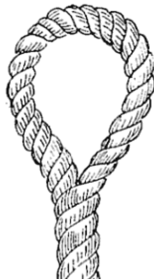
FIG. 90 B.—Flemish eye (complete).
