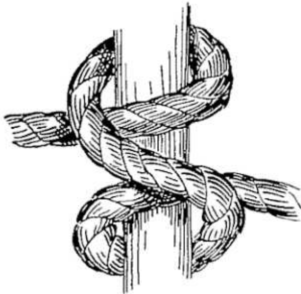
FIG. 36 A.—Clove hitch or builder's hitch (tying).
