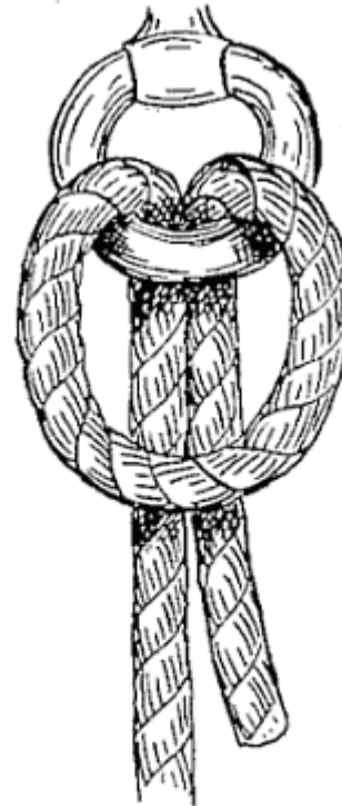
FIG. 31.—Lark's head with toggle (A) withdrawn.
